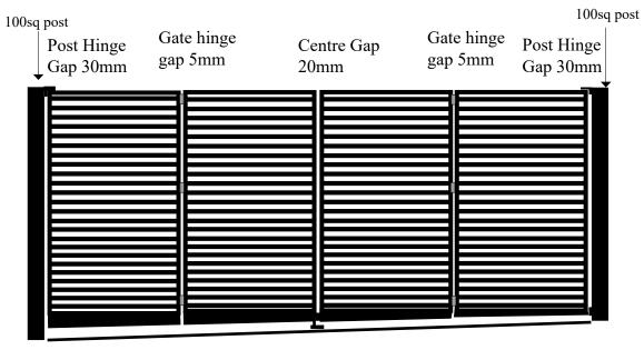
Post Height -Top hinge allowance 25mm Bottom hinge and sproket allowance 60mm
